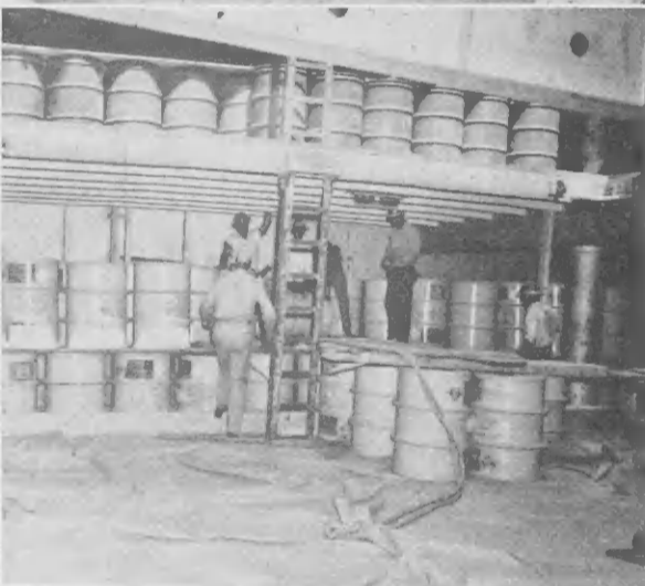
USING THE new bulk Ethyl system where the compound is pumped from storage tanks to weigh tanks, tedious jobs, above, and hazardous ones, left, have been eliminated.
